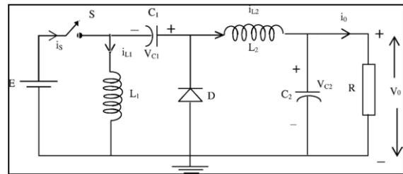
Fig. 2: Circuit diagram of Luo converter
