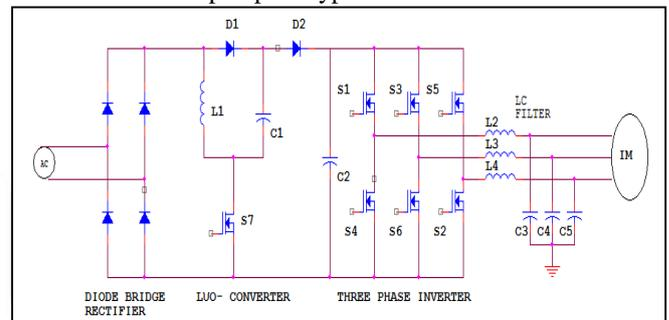
Fig. 1: Circuit Diagram of proposed System.
