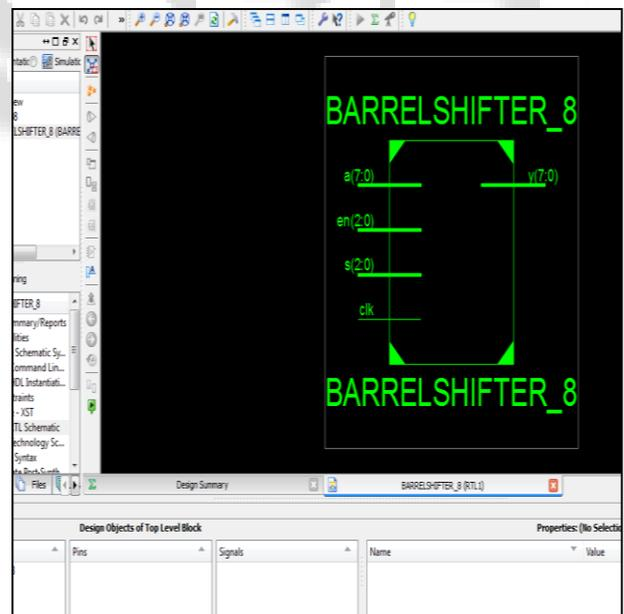
Fig. 4: RTL view of 8 bit barrel shifter
