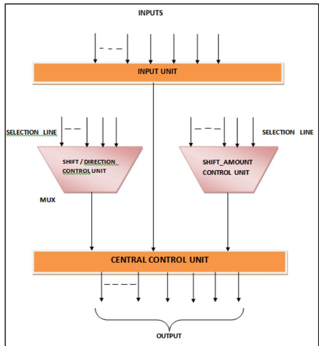
Fig. 3: Proposed block diagram of barrel shifter
