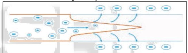
Fig. 5: Discharge of charge as polymer jet dries
