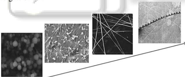
Fig. 7: SEM of different concentrations of polymer solution
