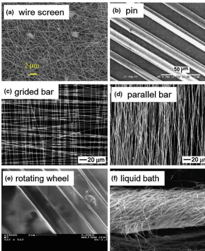
Fig. 9: Types of collectors
