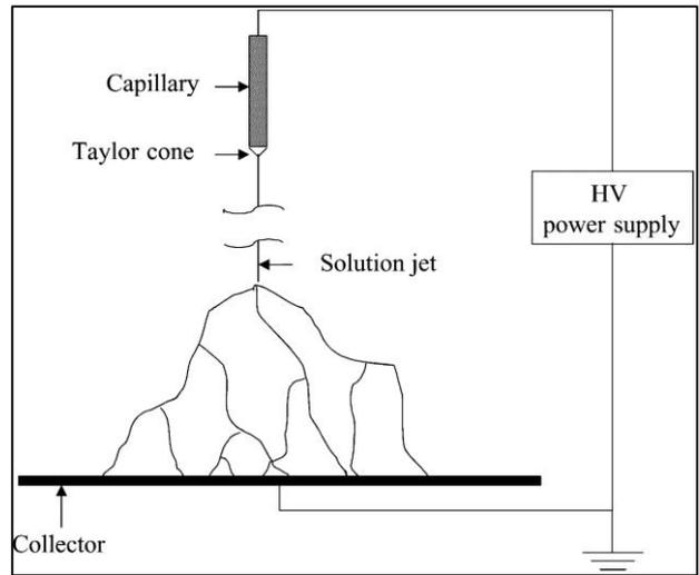
Fig. 3: Process of electro Spinning
