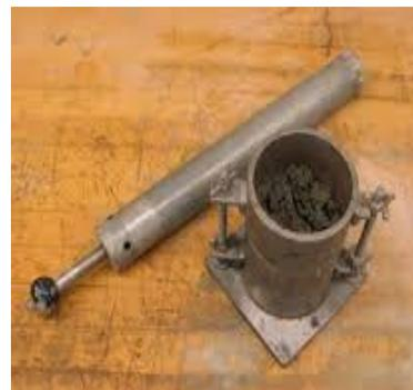
Fig. 3: Proctor test on clay soil.
