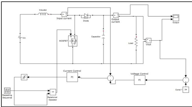
Fig. 7: Simulink model of closed loop boost converter with voltage and current control
