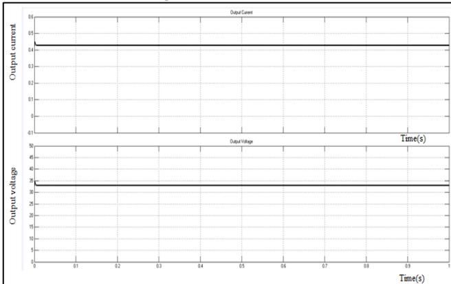
Fig. 8: Output waveforms of closed loop boost converter with voltage and current control
