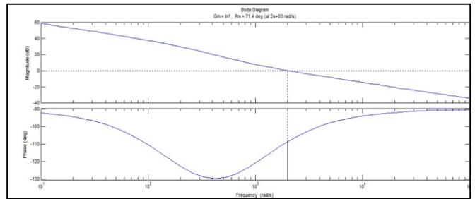
Fig.4 Bode plot for open loop transfer function of voltage loop
