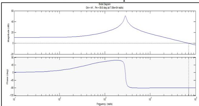
Fig. 3: Bode plot for open loop transfer function of current loop
