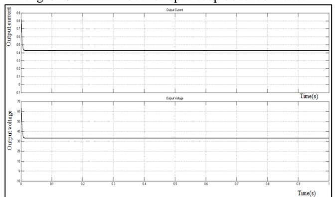
Fig. 6: Output waveforms of open loop boost converter
