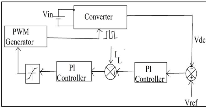
Fig. 2: Closed Loop Controlled Boost Converter
