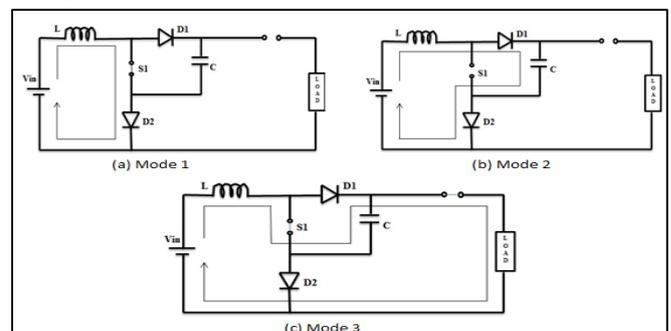
Fig. 3: Operating modes of modified boost converter
