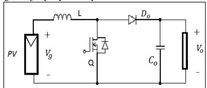
Fig. 1: Conventional boost converter [4]
