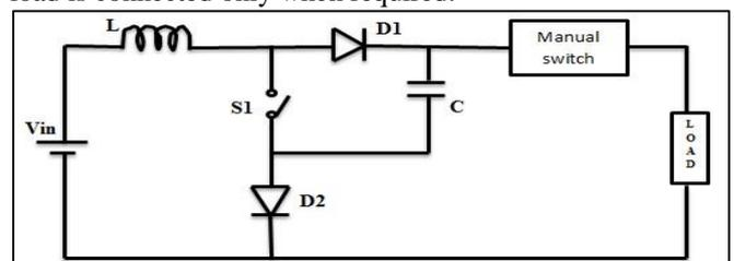
Fig. 2: Proposed boost converter
