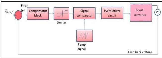
Fig. 4: Basic voltage control loop of the proposed converter [2]
