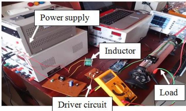
Fig. 7: Experimental setup of the proposed converter
