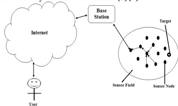
Fig. 1: Architecture of Sensor Network
