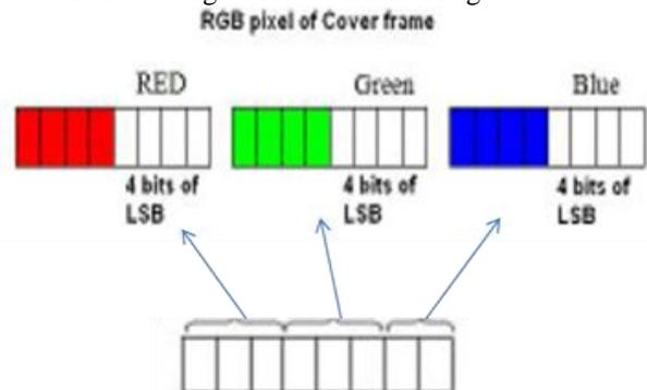
Fig. 7: LSB Shifting for RGB component of image.
