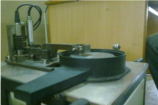
Fig. 10: shows pin-on-disc wear testing machine
