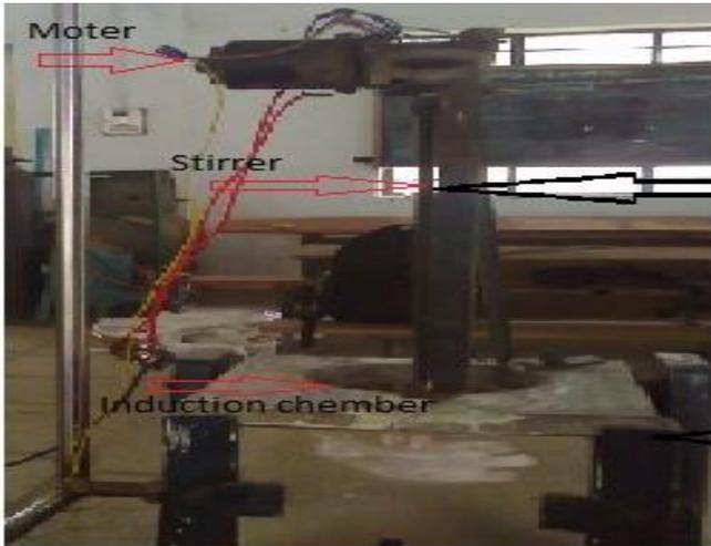
Fig.1: Shows Stir Casting setup
