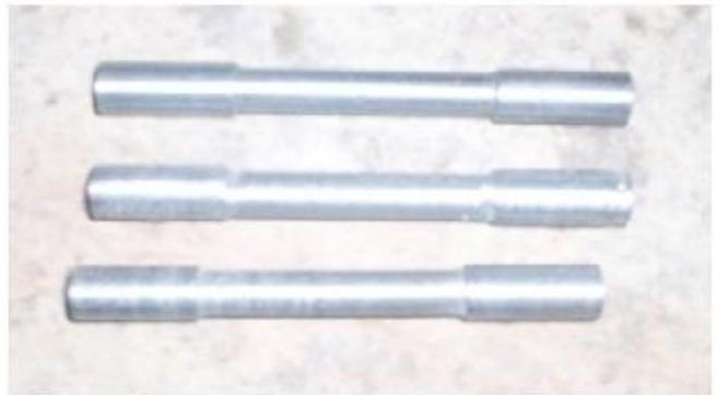
Fig. 4: Tensile Test Specimen after Machining
