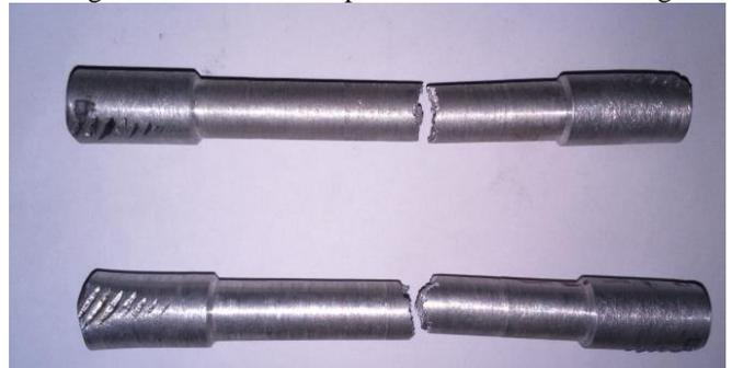
Fig. 5: Tensile Test Specimen after Testing
