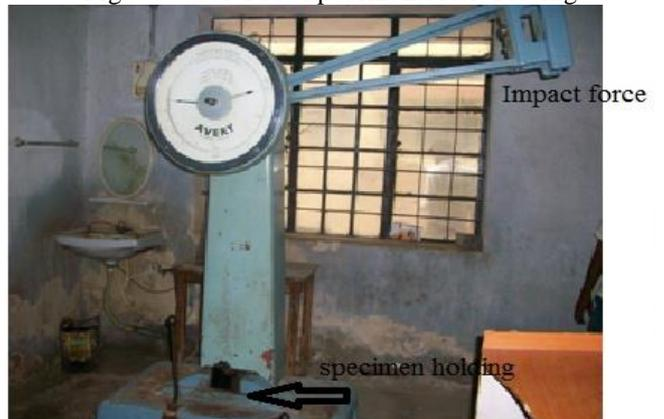
Fig. 8: Charpy Machine for Impact Test
