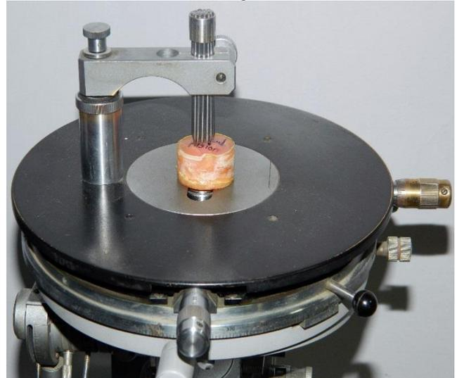
Fig. 4: Vicker's Microhardness Tester
