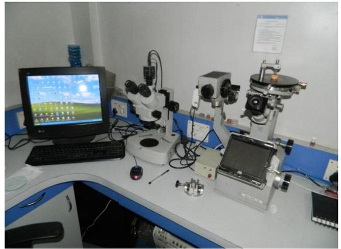
Fig. 3: Vicker's Micro hardness Tester
