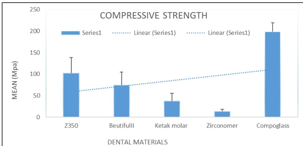
Fig. 5: Error bar chart illustrates the mean compressive strength and standard deviation
