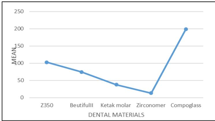
Fig. 6: Mean Compressive strength [MPa]
