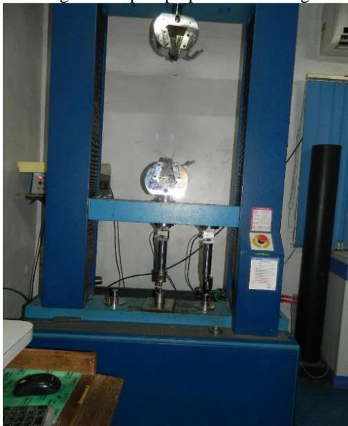
Fig. 2: Universal Testing Machine for compressive and flexural strength
