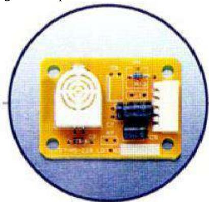
Fig. 5: Humidity Sensor Module
