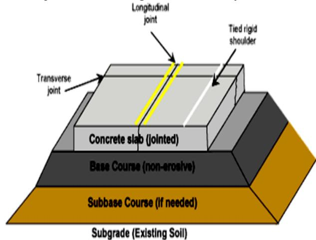
Fig. 1: shows the different layers of rigid Cement is the most important component of concrete, which is working in combination of the mix materials and increases the strength of concrete. The 75 % of concrete mix material is Aggregate. It is also playing important role in construction works, especially in concrete.
