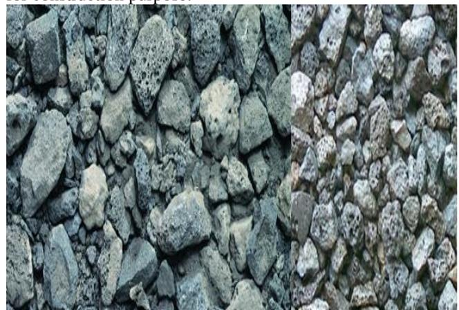
Fig. 6: Shows the sample of course Steel slag
