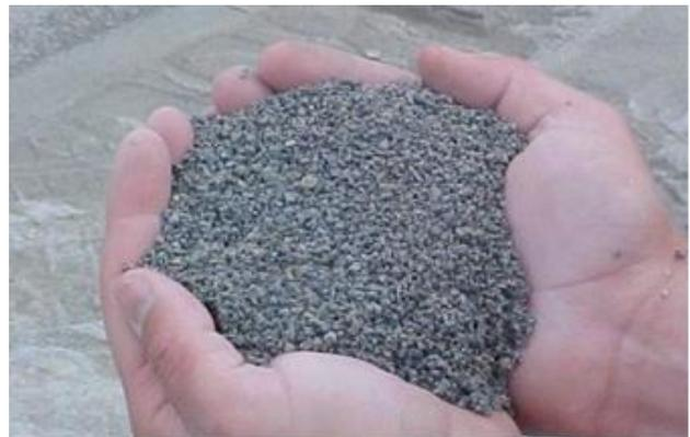
Fig. 4: shows fine Aggregates passing of 4.75 mm sieve
