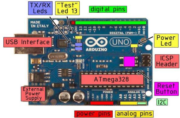
Fig. 4: Arduino Micro Controller
