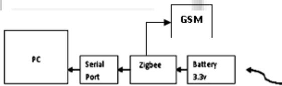
Fig. 2: Receiver Section
