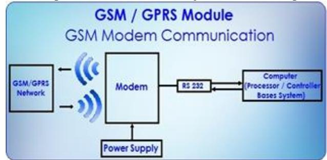
Fig. 6: Block Diagram of GSM Modem Communication
