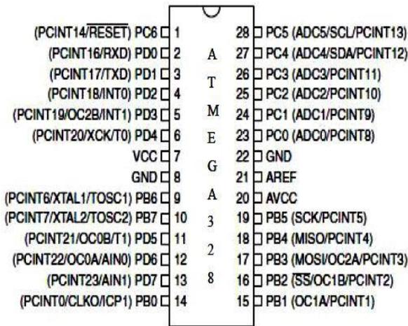
Fig. 5: Pin Diagram of ATmega328 Microcontroller
