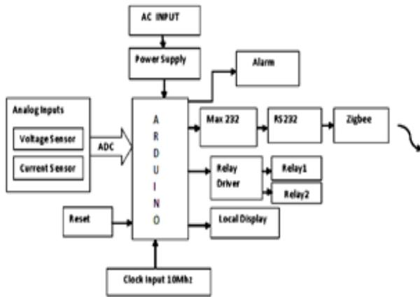
Fig. 1: Transmitter Section
