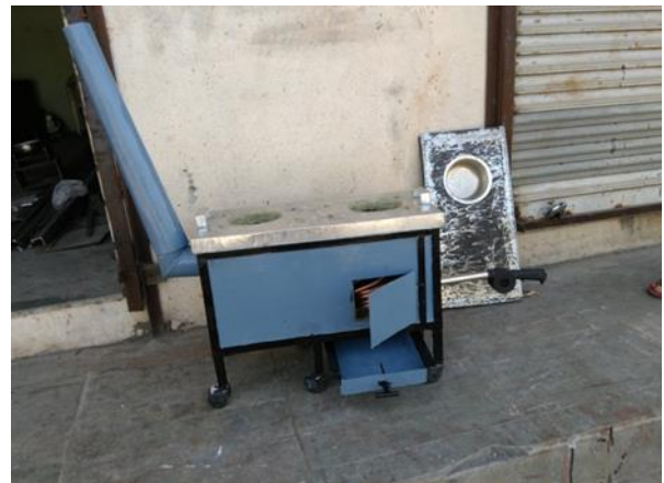
Fig. 8: Complete construction of chulha
