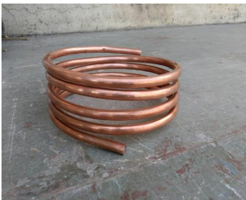
Fig. 7: Copper Tubing of chulha
