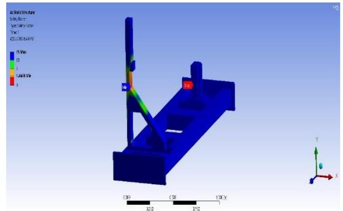
Fig. 2: Analysis of mounting bracket
