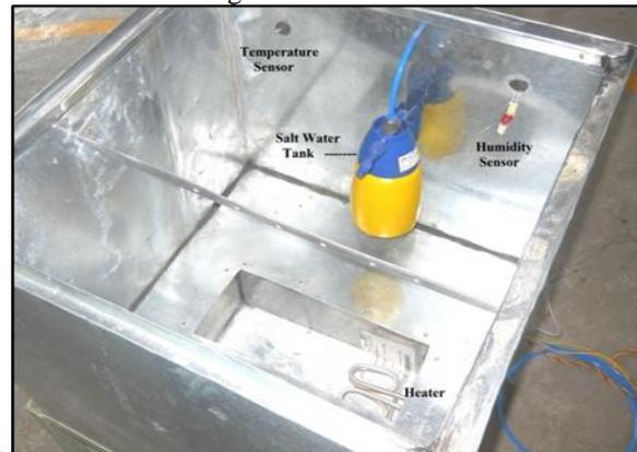
Fig. 3: Internal View of G.I. Chamber
