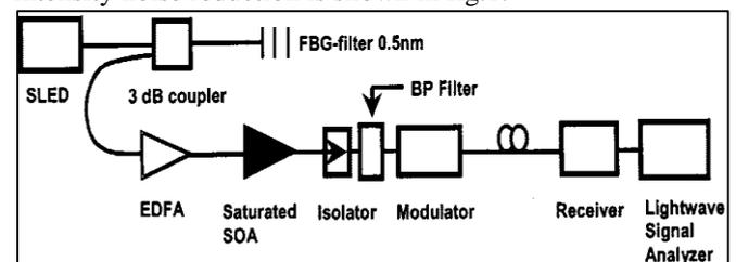
Fig. 1: Experimental setup for intensity noise reduction.
