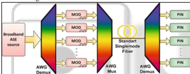
Fig. 2: Operating principle of spectrum-sliced WDM PON system
