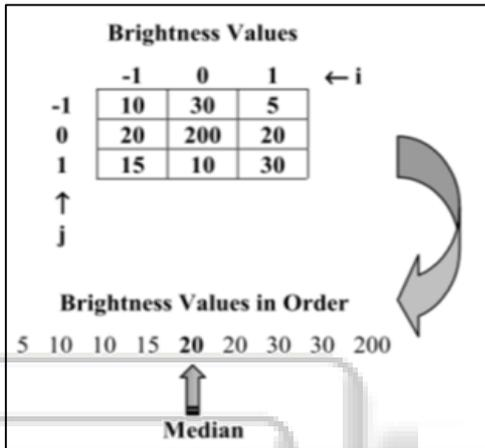
Fig. 2: example of median filter.
