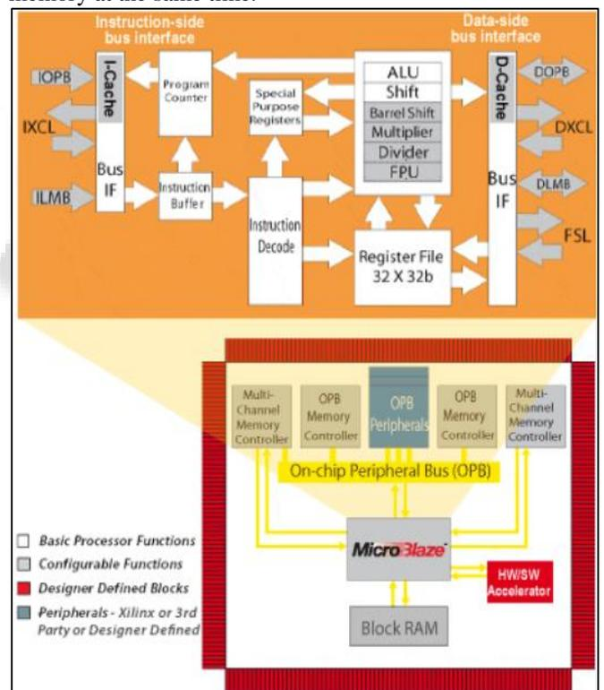
Fig. 1: A view of a Micro Blaze system
