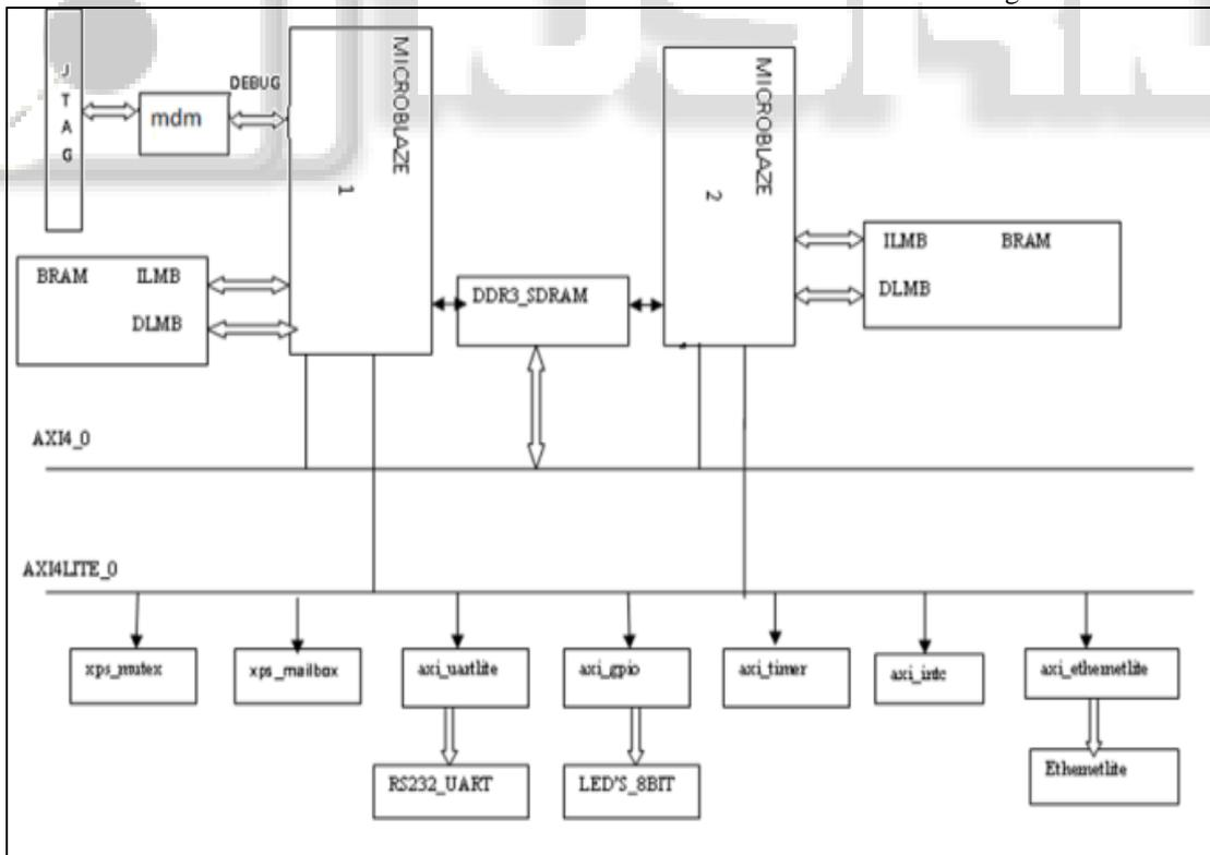
Fig. 4: Multi soft core architecture
