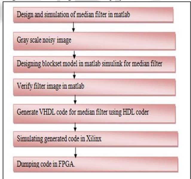
Fig. 6: Flow diagram for design and implementation of median filter in FPGA in HDL coder
