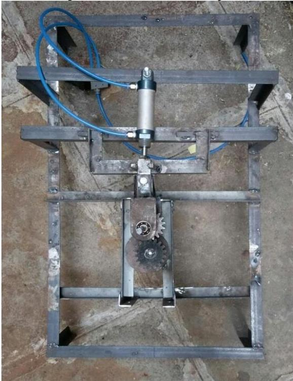
Fig. 4: Experimental Setup for Gear Burnishing
