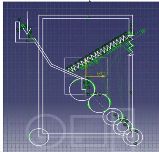
Fig. 1: Layout sketch of Automatic Pallet carrier For Small Workshop
