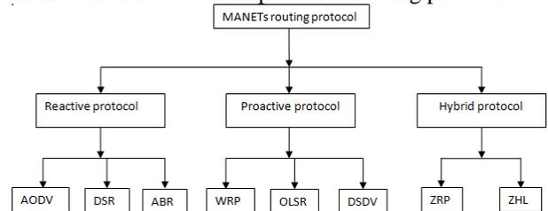
Fig. 2: Basic routing protocols of MANET
