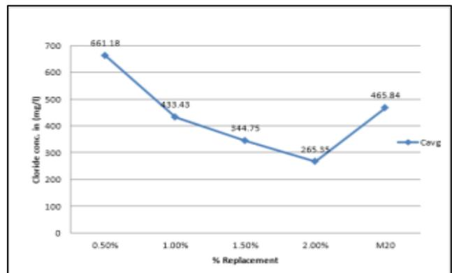
Fig. 7: Variation of chloride concentration
