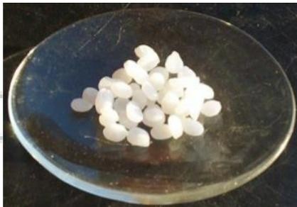
Fig. 4: Sodium hydroxide pallets
