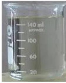
Fig. 3: Sodium Silicate Solution
