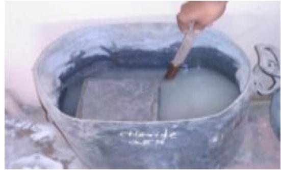
Fig. 5: Cubes kept for chloride attack
