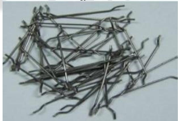
Fig. 2: Steel fibres
