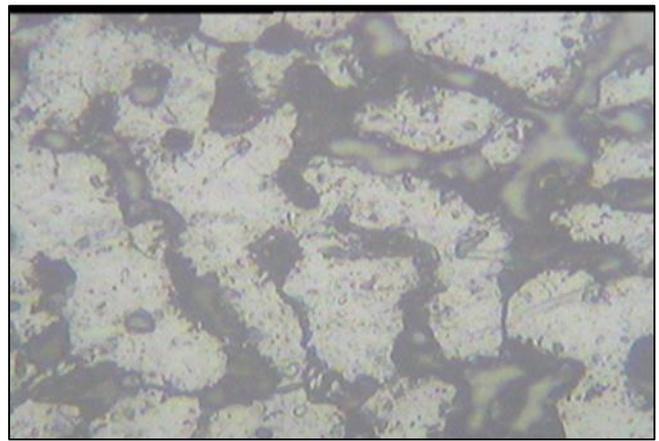
Fig. 1(b): Microstructure of Al - 25 Zn-2.5 Cu- 9 % SiC
