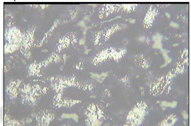
Fig. 1(c): Microstructure of Al - 25 Zn-2.5 Cu- 12 % SiC
