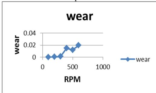
Fig. 3: Variation of wear with rpm
