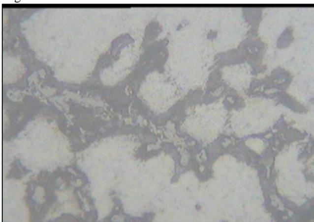
Fig. 1(a): Microstructure of Al - 25 Zn-2.5 Cu- 6 % SiC
