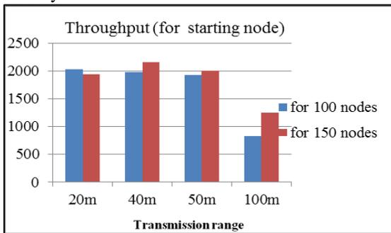
Fig. 12: Throughput for the starting (0<sup>th</sup>) node
