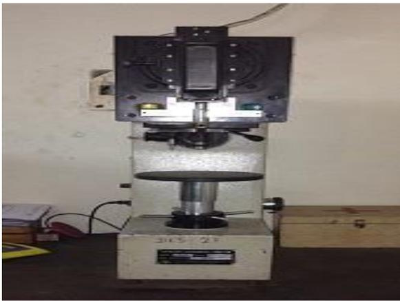
Fig. 5: Vickers hardness tester
