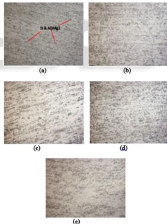
Fig. 4: Microstructure Of (A) Route A (B) Route Ba (C) Route Bc (D) Route C (E) Without ECAP
