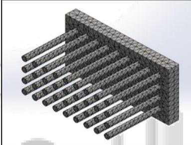
Fig. 6: Mesh Generation (Circular Fin)
