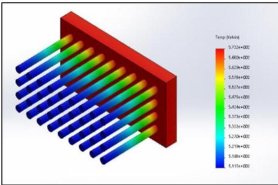
Fig. 12: Circular Fin (Aluminum Alloy 1060)
