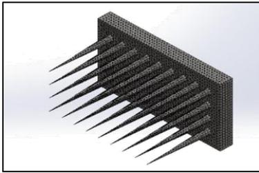
Fig. 4: Mesh Generation (Tapper- Fin)
