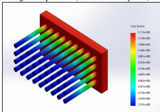
Fig. 11: Circular Fin (Alloy Steel)
