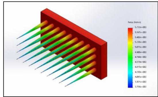
Fig. 7: Tapper fin(Alloy Steel)
