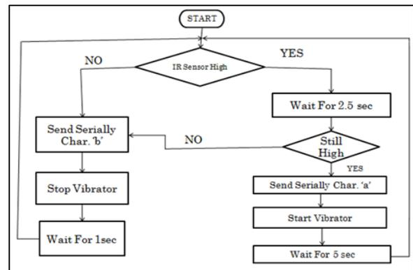
Fig. 5: Transmitter flow chart
