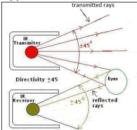
Fig. 3: Principle of IR sensor
