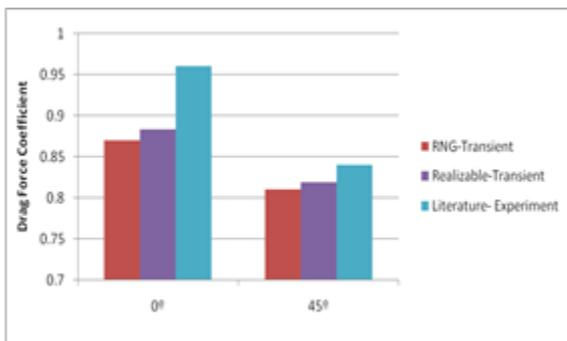
Fig. 4: Comparison of drag force value by various simulations
