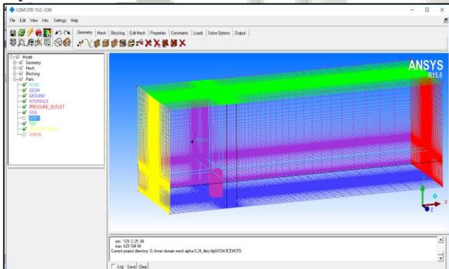
Fig. 3: Mesh of inner core surface.
