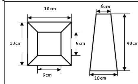
Fig. 1: Plan and Elevation view of the model
