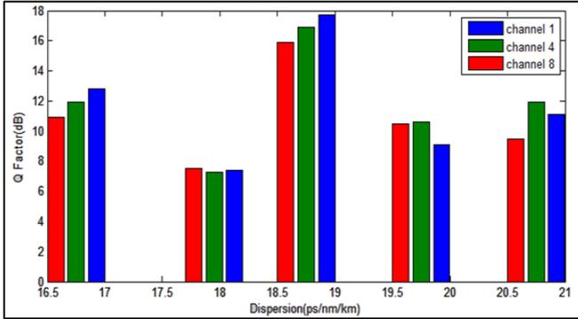
Fig. 4: Effect of chromatic dispersion on Q factor
