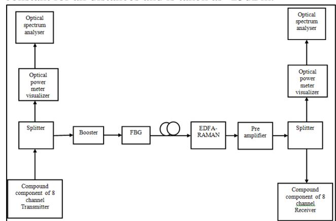
Fig. 1: Block diagram for simulation setup
