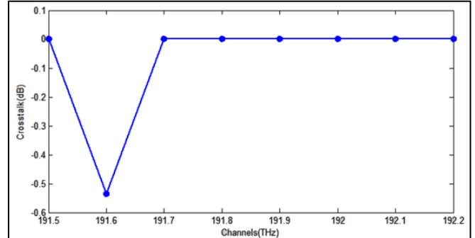
Fig. 5: Crosstalk between 8 channels at 100GHz channel spacing with NRZ pattern
