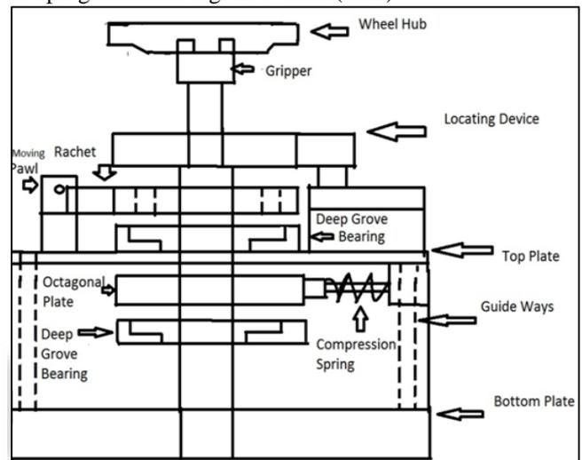
Fig. 1: Conceptual Design of SPM
