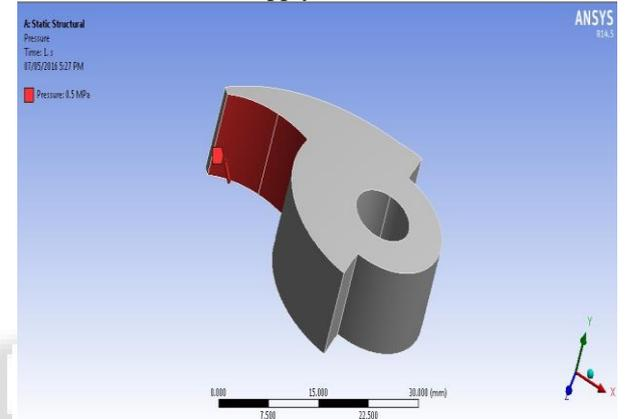
Fig. 11: Total Pressure Apply On Pawl Teeth
