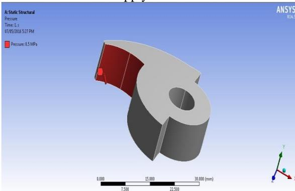
Fig. 6: Total Pressure Apply On Pawl Teeth
