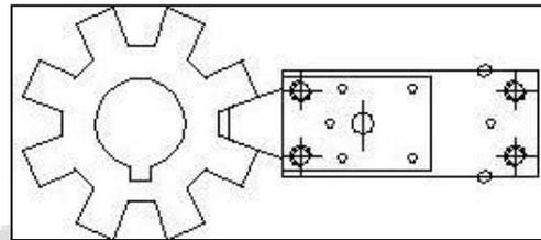
Fig. 4: Indexing Plate with Locating Device
