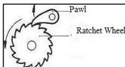
Fig. 2: Schematic Diagram of Ratchet and Pawl [14].
