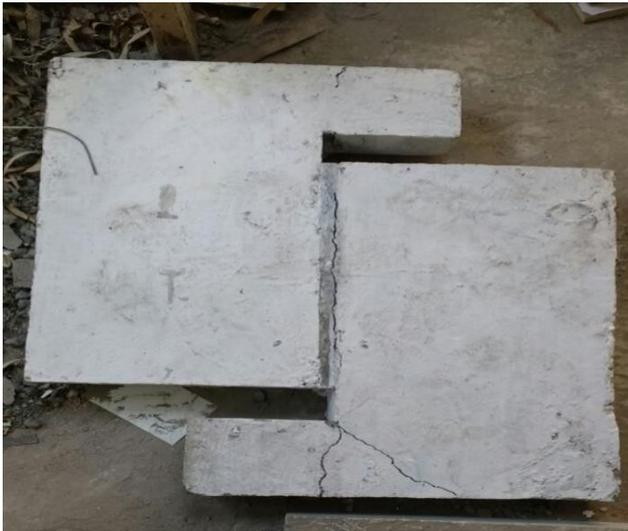
Fig. 6: Failure in Connection
