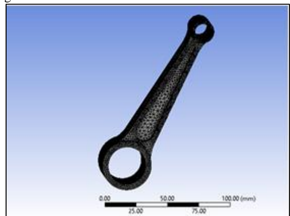
Fig. 5: Meshing applied on connecting rod model
