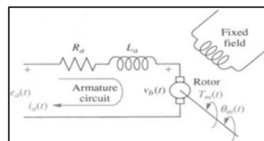
Fig. 1: DC Motor System
