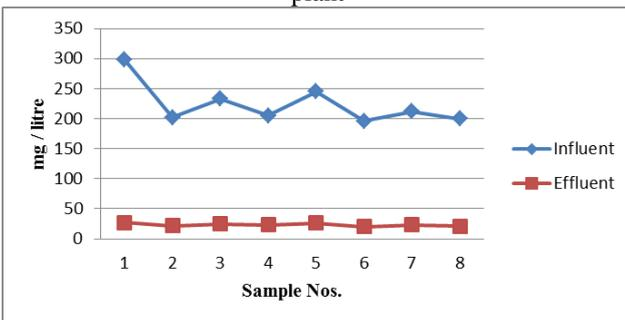
Fig. 5: TSS concentrations of influent and effluent of the Bharwara UASB plant
