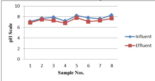
Fig. 2: pH Variation b/w influent and effluent of the Bharwara UASB plant
