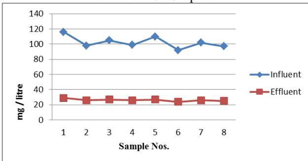
Fig. 3: BOD5 of influent and effluent of the Bharwara UASB plant
