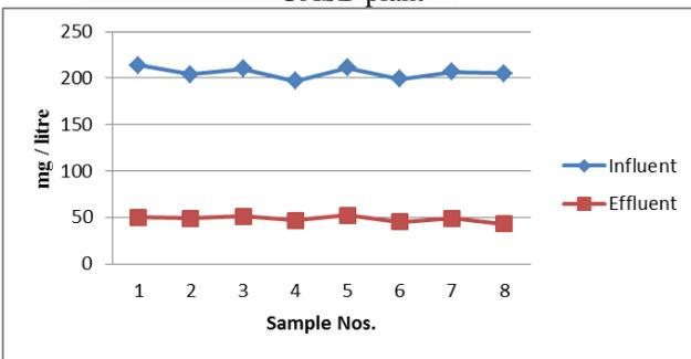
Fig. 4: COD of influent and effluent of the Bharwara UASB plant
