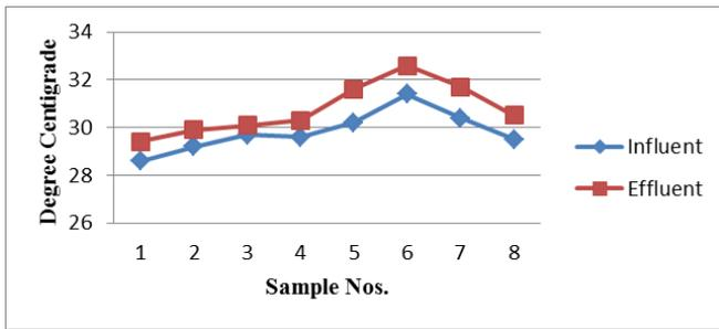
Fig. 1: Temperature Variation b/w influent and effluent of the Bharwara UASB plant
