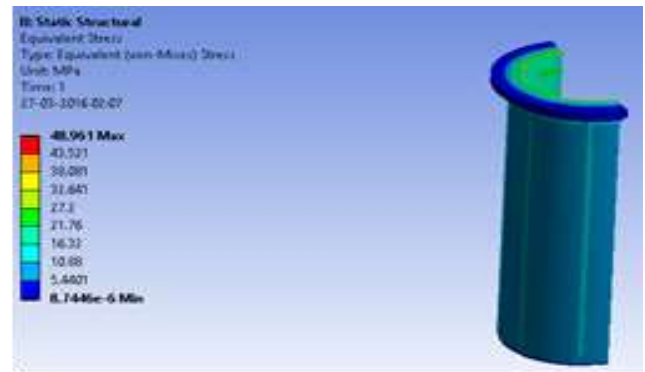
Fig. 8: Equivalent stress on optimized liner design
