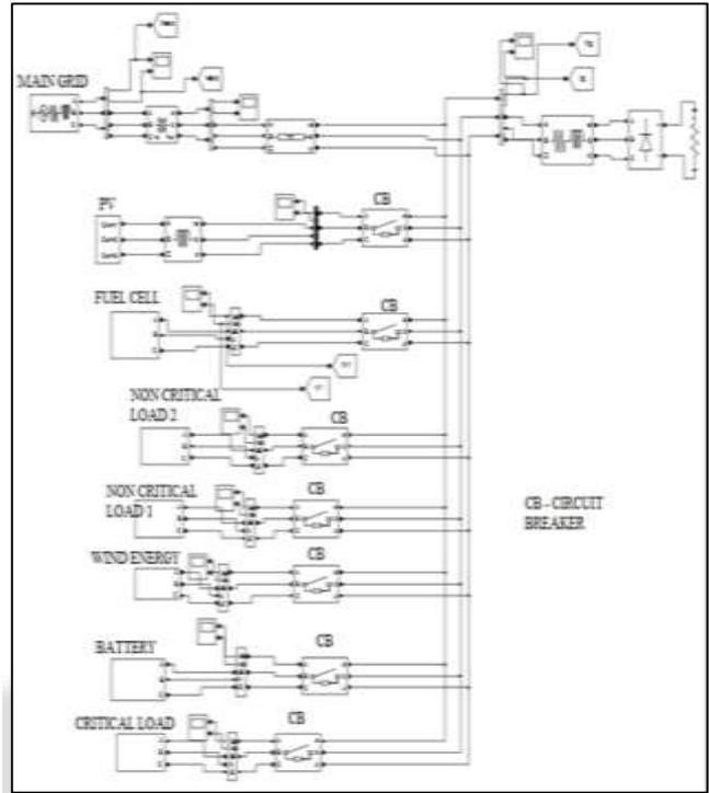
Fig. 5: Simulation circuit of Micro Grid
