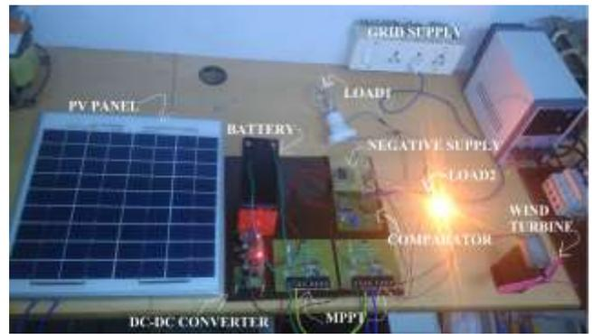
Fig. 13.1: Prototype hardware model(Islanding mode)
