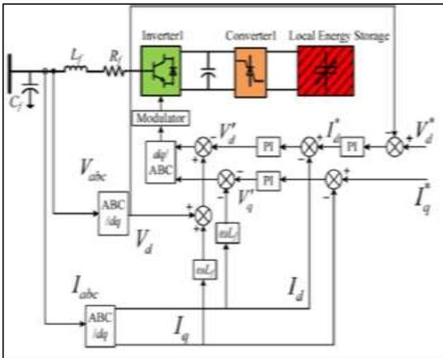
Fig. 4: Control circuit for LES (Islanding mode)
