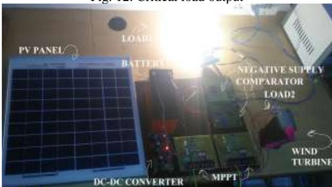
Fig. 13: Prototype hardware model(Grid connected)
