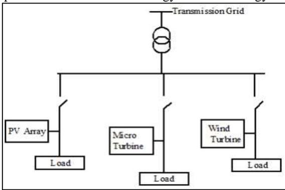
Fig. 1: Basic module of micro grid
