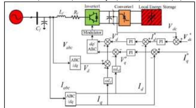
Fig. 3: Control circuit for LES (Grid connected mode)
