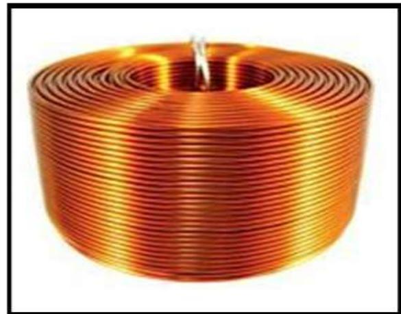
Fig. 4: Receiver coil
