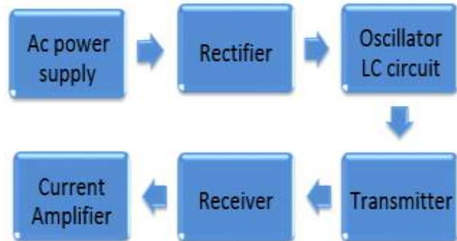
Fig. 1: Block diagram of wireless charger
