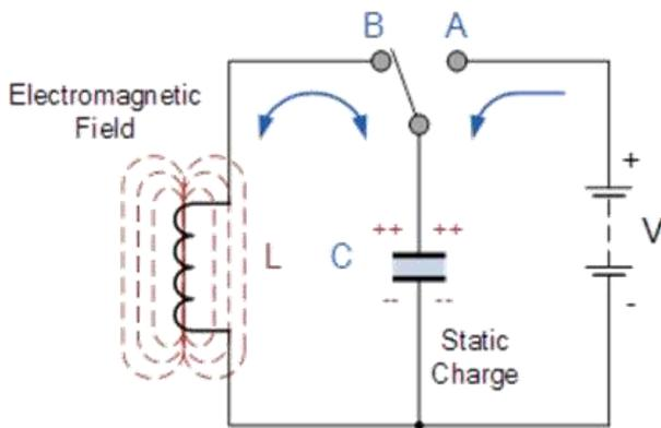
Fig. 5: Basic oscillator tank circuit
