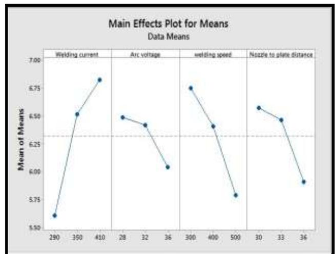
Fig. 4: Main Effects Plot of Penetration
