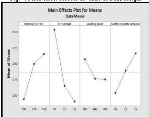
Fig. 8: Main Effects Plot of Bead Height
