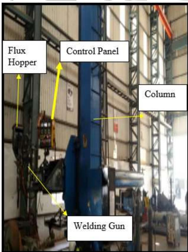
Fig. 1: Single wire submerged arc welding
