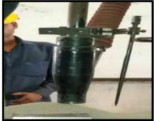
Fig. 2: SAW welding operation
