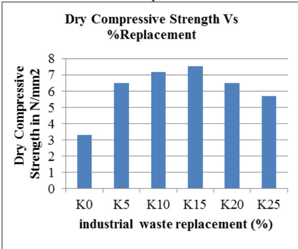
Fig. 4: dry compressive strength Vs % replacement
