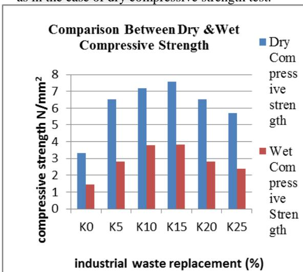
Fig. 5: comparison between wet and dry compressive Strengths
