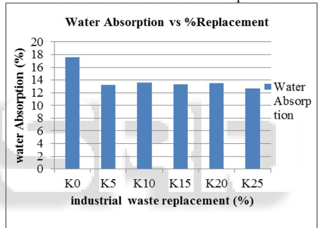
Fig. 3: Water Absorption Vs % Replacement
