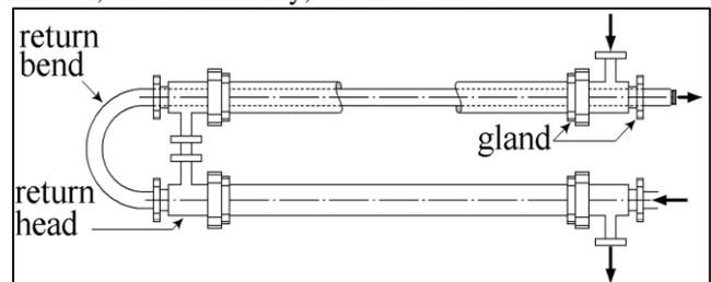
Fig. 2: Double Pipe Heat Exchanger
