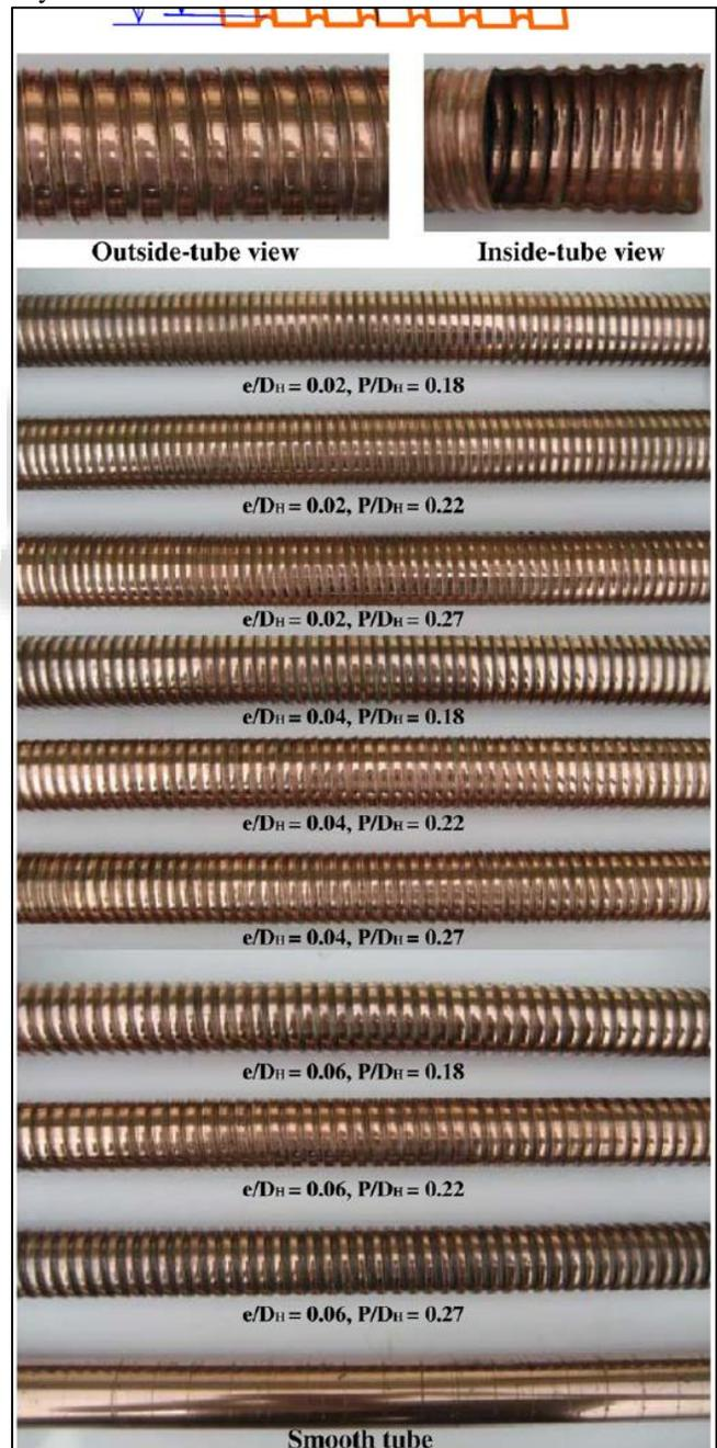
Fig. 4: Photograph of helically-corrugated/smooth tube
