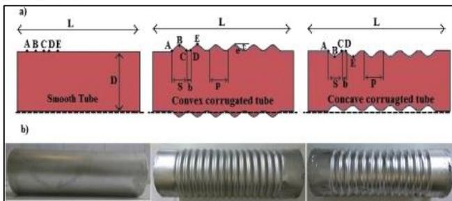
Fig. 3: Schematic diagram of smooth tubes and corrugated tubes
