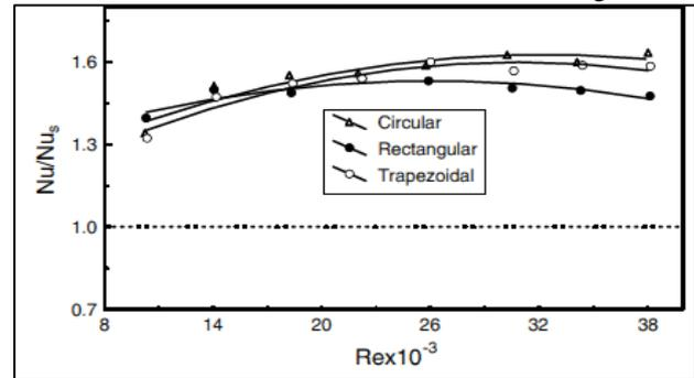
Fig. 5: Variation of Nusselt number ratio with Reynolds number for different grooved tubes
