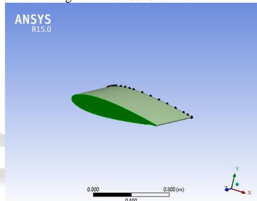
Fig. 2: NACA0018 3D model
