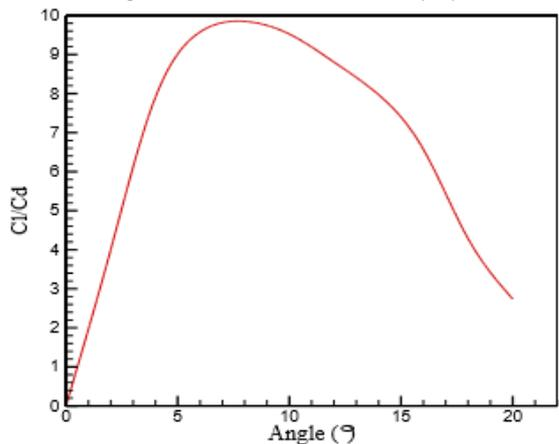
Fig. 6: C<sub>l</sub>/C<sub>d</sub> variation with AOA (α<sup>0</sup>)
