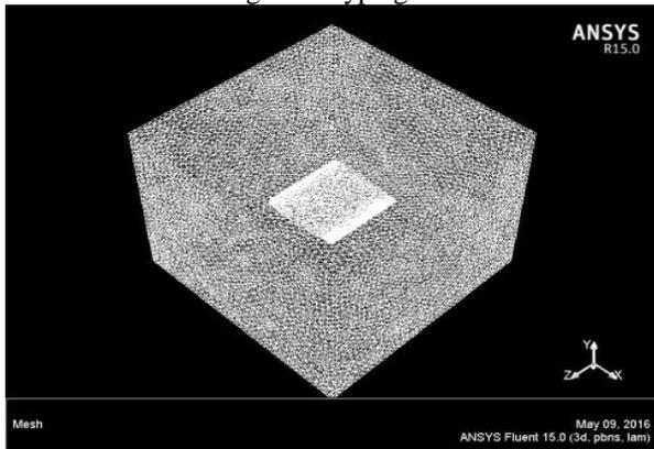
Fig. 4: Highly Dense Mesh Near Airfoil
