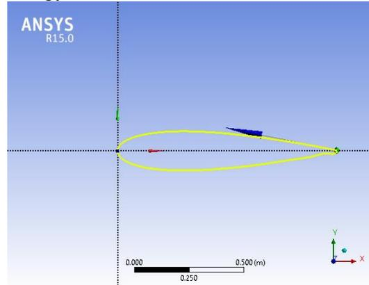
Fig. 1: NACA0018 2D model
