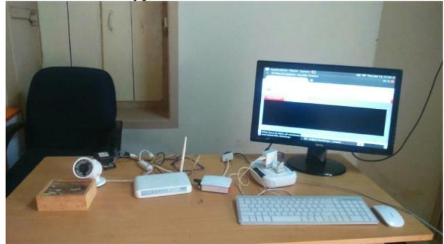
Fig. 2: Raspberry pi setup with camera module
