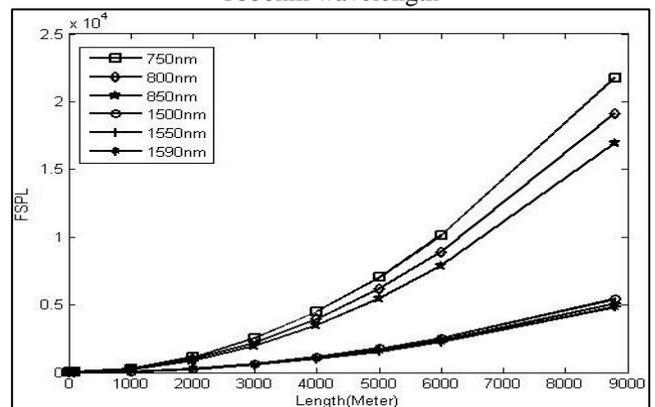
Fig. 2: FSPL v/s transmission distance for FSO system in haze weather at (a) 750, 800 & 850nm (b) 1500, 1550 & 1600nm wavelength
