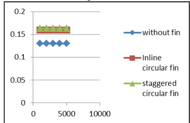
Fig. 4: Reynold no vs friction factor in different types of fin arrangements
