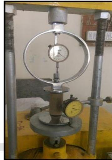
Fig. 4: Experimental set up of UCS
