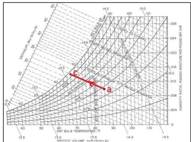
Fig. 1: Indirect Evaporative Cooling
