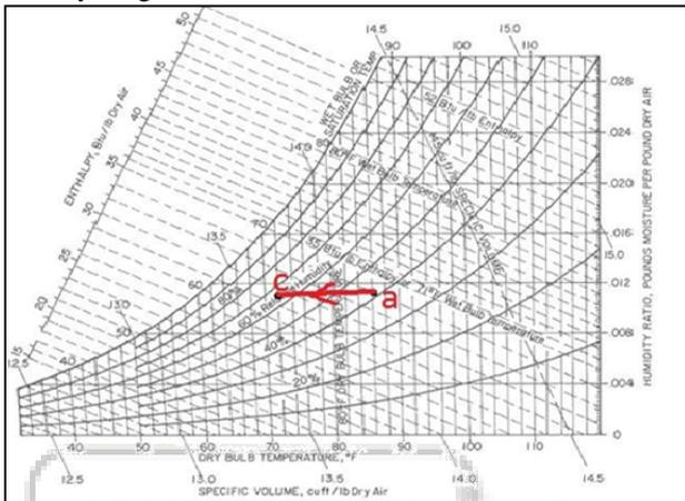
Fig. 2: Direct Evaporative Cooling
