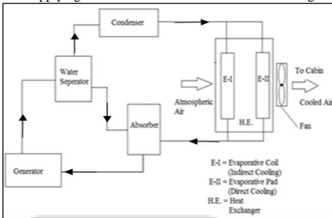
Fig. 5: Block diagram of VAS Vapour Assisted Air Cooler
