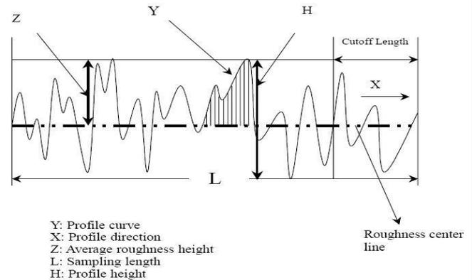
Fig. 1: Surface Roughness Graph
