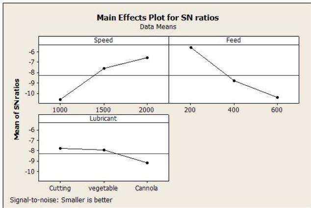
Graph 2: Response Graph of three machining parameters for S/N ratio for SR
