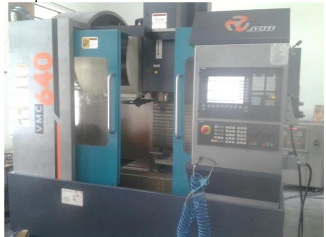
Fig. 2: CNC Milling Machine
