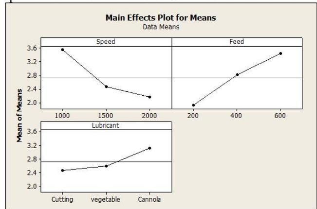
Graph 1: Response Graph of three machining parameters for mean for SR
