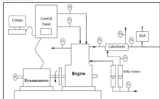
Fig. 1: Line diagram of experimental setup
