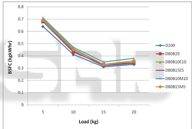
Fig. 2: Brake Specific Fuel Consumption Vs Load
