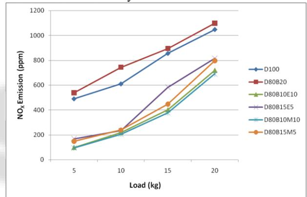
Fig. 7: Oxides of Nitrogen content Vs. Load
