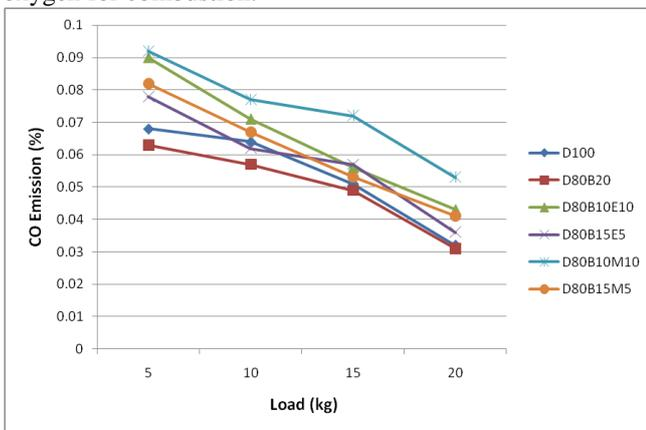
Fig. 4: Carbon monoxide content Vs Load
