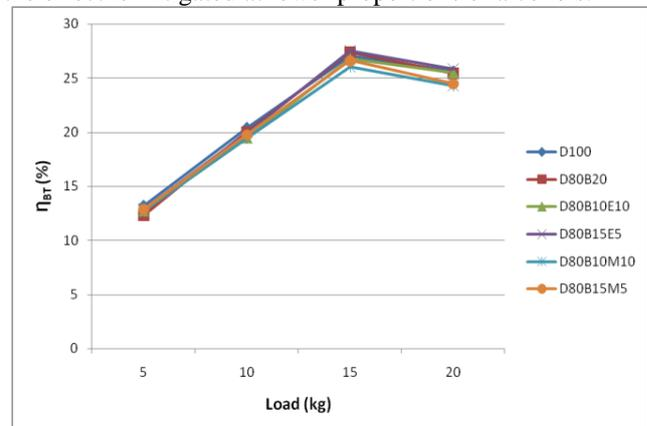
Fig. 3: Brake Thermal Efficiency Vs Load
