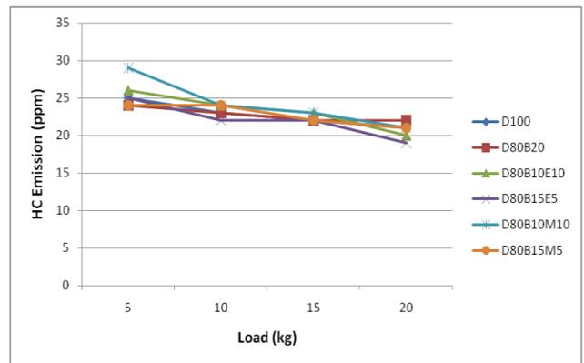
Fig. 6: Hydrocarbon content Vs Load
