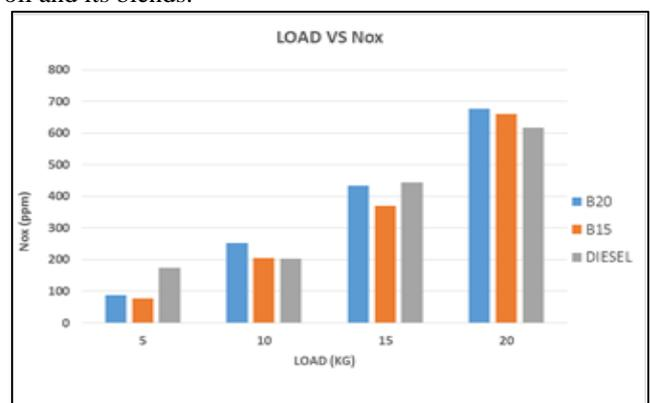
Fig. 7: Load vs Oxides of Nitrogen
