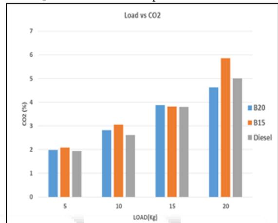
Fig. 6: Load Vs CO<sub>2</sub> emission
