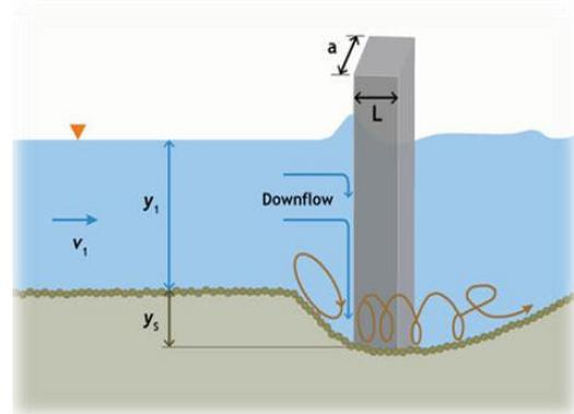
Fig. 2: Scour at Pier Foundation
