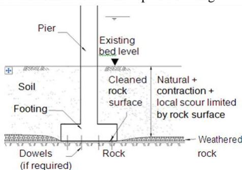
Fig. 3: Spread footing on sound rock.
